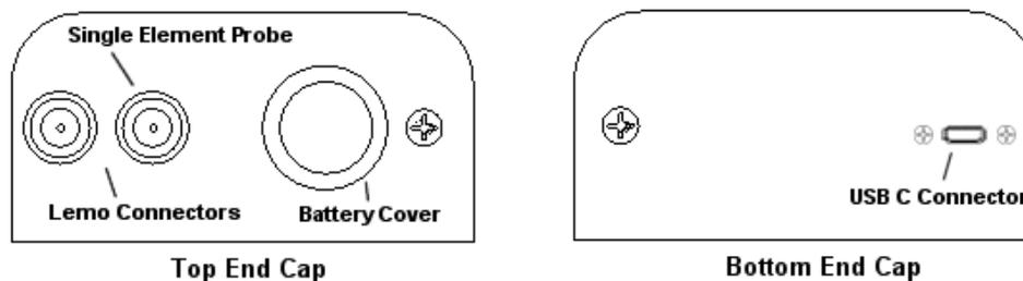
The top end cap is where all connections are made to the **ZX-5 DL**. The diagram above shows the layout and description of the connectors:
