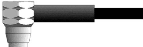
The Transducer is the “business end” of the **ZX-5 DL**. It transmits and receives ultrasonic sound waves that the **ZX-5 DL** uses to calculate the thickness of the material being measured. The transducer connects to the **ZX-5 DL** via the attached cable, and two coaxial connectors. When using transducers manufactured by Dakota Ultrasonics, the orientation of the dual coaxial connectors is not critical: either plug may be fitted to either socket in the **ZX-5 DL**.
