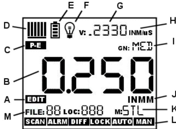
The **ZX-5 DL** uses a custom glass LCD backlit low temperature display for use in a variety of climate conditions. It contains graphic icons, as well as both 7 and 14 segment display areas. Let's take a closer look and what all these things are telling us:
