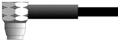
The Transducer is the “business end” of the **ZX-5**. It transmits and receives ultrasonic sound waves that the **ZX-5** uses to calculate the thickness of the material being measured. The transducer connects to the **ZX-5** via the attached cable, and two coaxial connectors. When using transducers manufactured by Dakota Ultrasonics, the orientation of the dual coaxial connectors is not critical: either plug may be fitted to either socket in the **ZX-5**.
