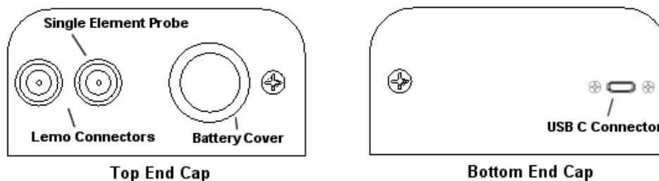
The top end cap is where all connections are made to the **ZX-5**. The diagram above shows the layout and description of the connectors:
