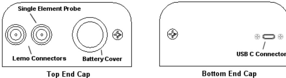
The top & bottom end panels are where all connections are made to the **CMX<sup>DL</sup>**. The diagram above shows the layout and description of the connectors:
