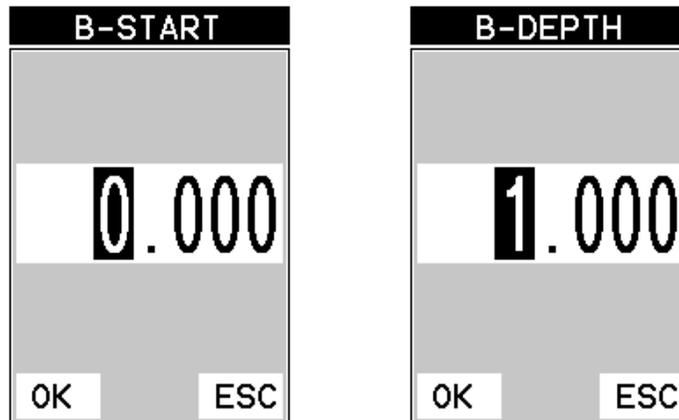
Alternatively, the **B-START** and **B-DEPTH** values can be changed using the **Digit Edit Box** as follows:
