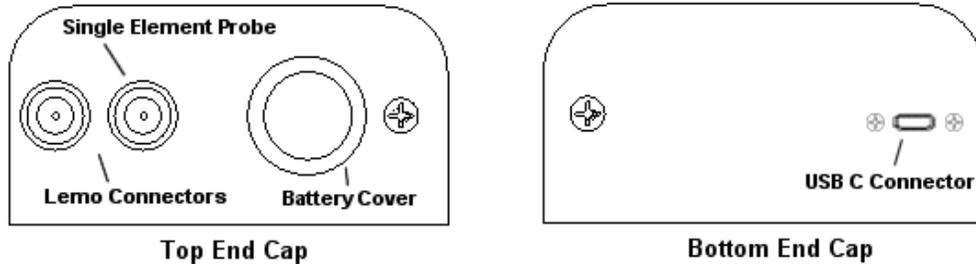
The top & bottom end panels are where all connections are made to the **CMX**. The diagram above shows the layout and description of the connectors:
