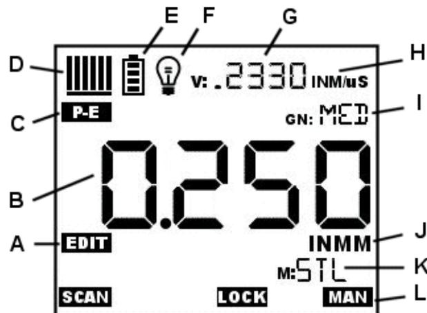
The **PR-9** uses a custom glass LCD backlit low temperature display for use in a variety of climate conditions. It contains graphic icons, as well as both 7 and 14 segment display areas. Let's take a closer look and what all these things are telling us:
