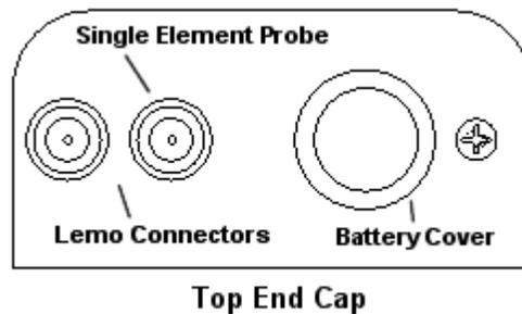
The top end cap is where all connections are made to the **PR-9**. The diagram above shows the layout and description of the connectors:
