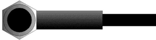
This is a top view of a typical transducer. Press against the top with the thumb or index finger to hold the transducer in place. Moderate pressure is sufficient, as it is only necessary to keep the transducer stationary, and the wear face seated flat against the surface of the material being measured.
