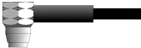
The Transducer is the “business end” of the **PR-9**. It transmits and receives ultrasonic sound waves that the **PR-9** uses to calculate the thickness of the material being measured. The transducer connects to the **PR-9** via the attached cable, and two coaxial connectors. When using transducers manufactured by Dakota Ultrasonics, the orientation of the dual coaxial connectors is not critical: either plug may be fitted to either socket in the **PR-9**.
