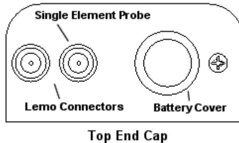
The top end cap is where all connections are made to the **ZX-2**. The diagram above shows the layout and description of the connectors:
